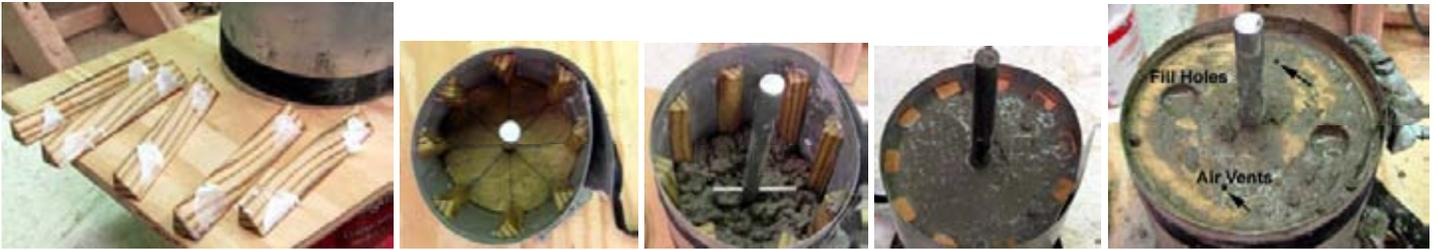
Remove the cylinder when you are comfortable that the concrete has cured sufficiently to be able to wire brush the teeth to expose the aggregate. Do not wire brush the V section of the teeth. Again, keep the end caps in place for about 24 hours until the concrete has cured enough to safely remove them without damaging the edges. Again, cover with a wet cloth and plastic and keep wet for curing.
