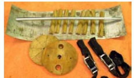
Insert T-1 pin in the center of shaft T-3, and push T-3 through the end cap V-1 so the radial lines are visible from the inside of the mold.
