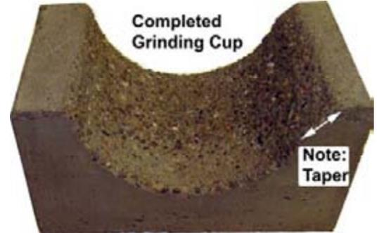
Remove the four sides of the mold when you are comfortable that the concrete is firm but soft enough to scrub to expose the aggregate. Make certain that you scrub from both sides toward the center so as not to damage the edges.
