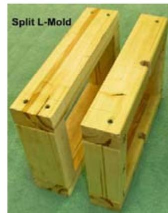
After the grinding cup has cured and following the registration marks, reassemble the bottom section of the mold around the grinding cup and leave 1 inch of the grinding cup extending beyond the back of wood frame. Place a screw eye on the top edge, i.e. the end with the taper.
