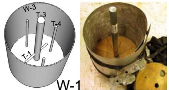
Fill the mold with concrete containing aggregate to about 1 inch from the top.
