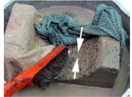
Reassemble the L-Mold and cut the mold into two sections at the cut line. Keep the bottom section of the mold as the holder for the grinding cup.
