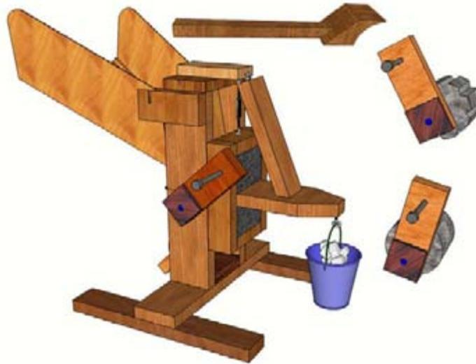
The Easy BioGrind® biomass grinder was designed to grind dry biomass and to accomplish a number of goals. The objectives were the flexibility to grind a wide variety of dry biomasses, low-cost, easy to build using mostly hand tools, easy to operate, easy to maintain and require no welding.
